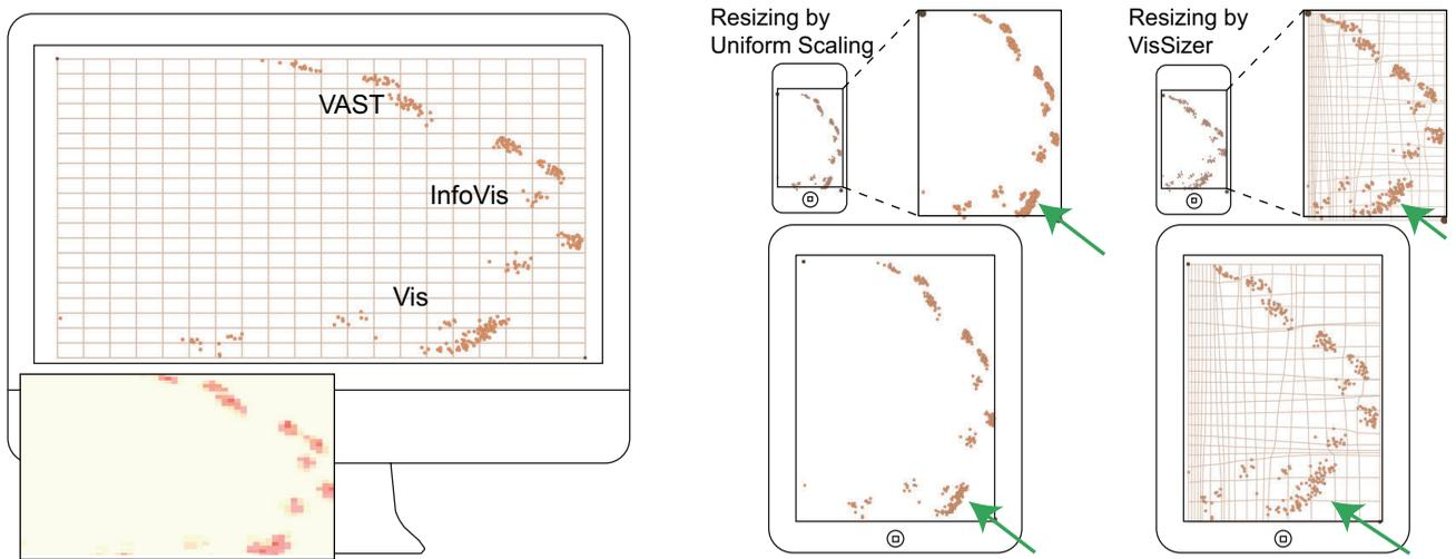
Fig. 8. Results created by resizing a scatterplot originally shown on a 21.5 inch display with  $1920 \times 1080$  pixels (left) to a 3.5 inch display with  $960 \times 640$  pixels and a 9.7 inch display with  $1024 \times 768$  pixels by uniform scaling (middle) and ViSizer (right). Through the judicious removal of white space, ViSizer assigns more space to important areas and maintains the overall pattern, thus showing the relationships among the points in clusters more clearly.
